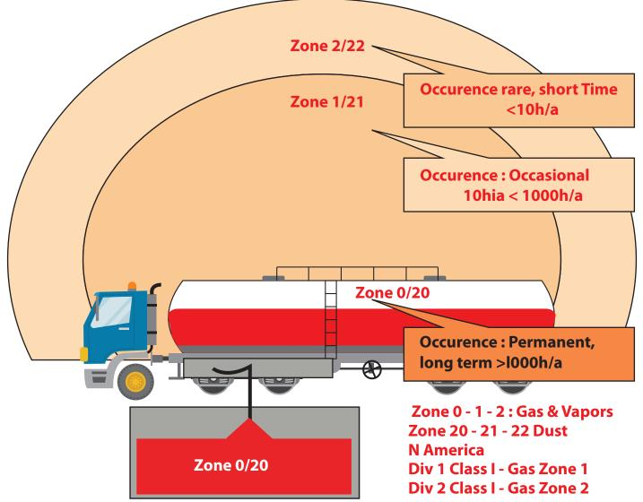
Hazardous areas are classified into zones based on an assessment of the frequency of the occurrence and duration of an explosive gas atmosphere, as follows:
