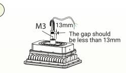
2. Tighten the hook with the fixture, at least 6x teeth need to be tighten, fix the M3 screw to prevent the hook loosening .
