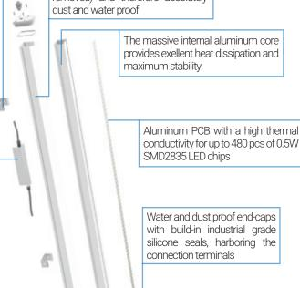
Internal high quality power driver contanining real Rubycon capacitors, Toshiba IC's and other high grade copmonents
